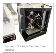
Optimized fittings and precut tubing ensure maximum reliability and instrument up-time.
