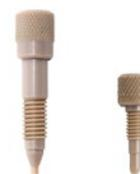
PEEKLoK™ UHPLC fittings are designed specifically for PEEKsil tubing: reliable, affordable, and easy to use, holding up to 22,000 psi; or up to 15,000 psi when used with ProDx trap columns.
