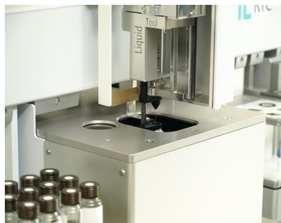
Figure 3: Centrifuge as part of automatic epoxidation.
